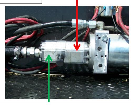
**Secondary Pump** – Delivers an additional 1.8 GPM <u>ONLY</u> when operating pressure is below 1,400 PSI. Maximum combined flow (Primary plus Secondary) at 1,400 PSI and below is approx. 5.5 GPM.
